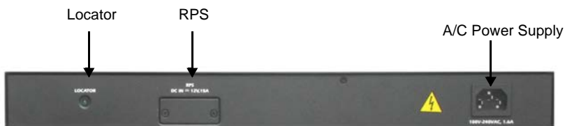
Figure 3-4. PowerConnect 5524/48/P Back Panel
